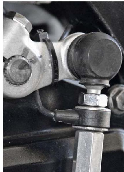
**1b. QSE Sensor under the bolt of shift arm**
