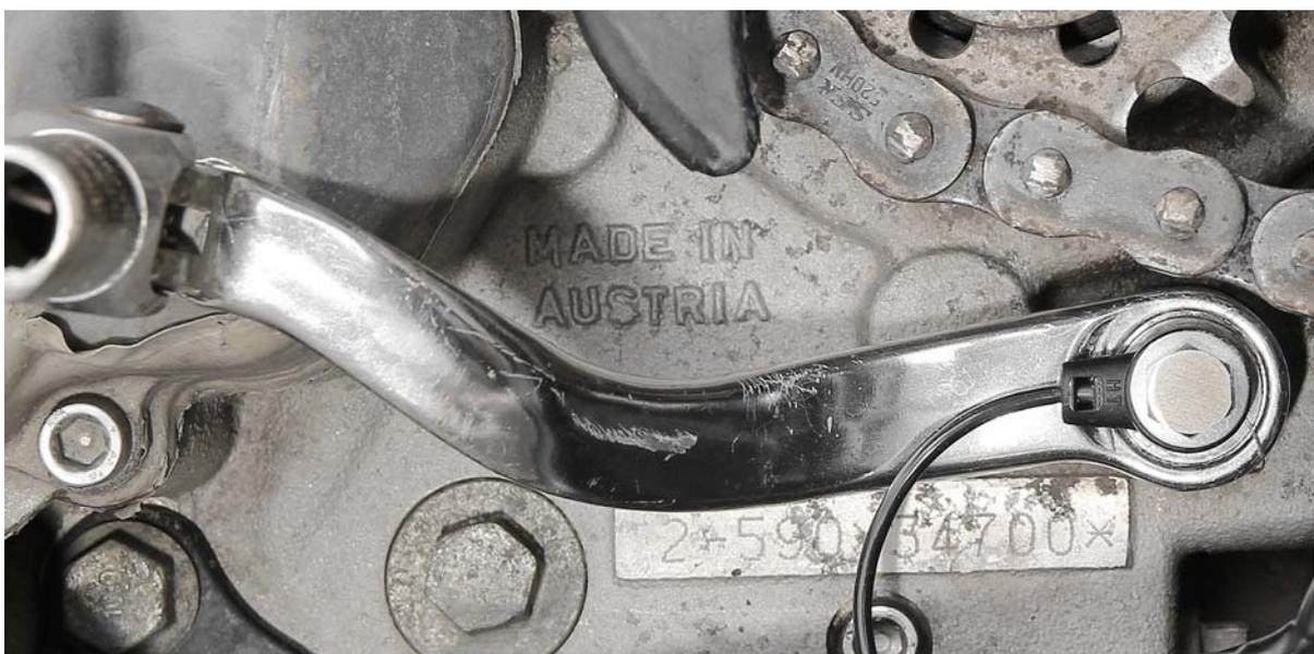
**1d. QSE Sensor under the bolt of shift lever (typically on off-road bikes)**
