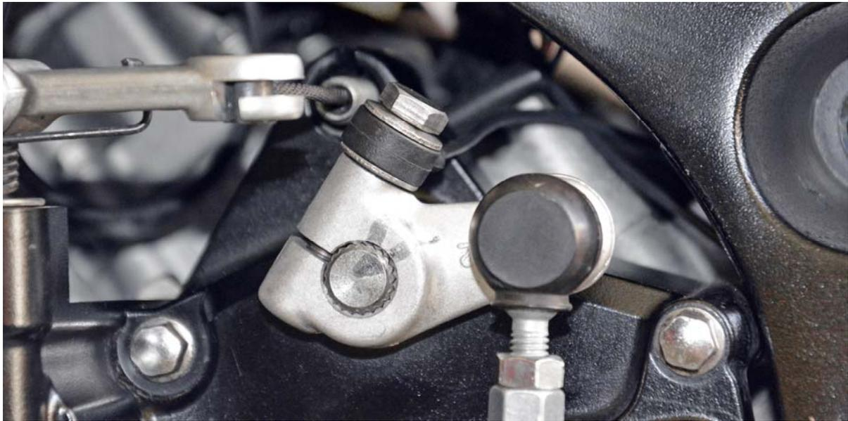
**1c. QSE Sensor under the bolt of gearbox shaft (typically on KTM bikes)**
